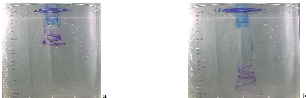
Fig. 2. Transport of blue and purple dyes from surface spots inside compound vortex ( H = 40 cm, \Omega = 180^\circ\text{revo} , R = 5.0 cm): a, b – t = 5, 15 s.
