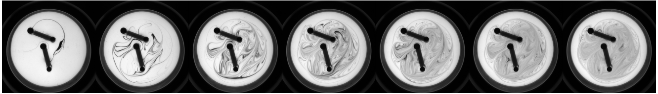
Figure 2: A time sequence of mixing for 0.1% solution of Carbopol EZ-3, which has a measured yield stress of 2.5 Pa. The time between images is 4 periods.
