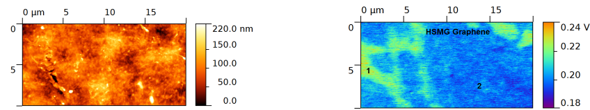
Fig. 1: Kelvin probe microscopy observation of the graphene membranes. Left - topography; right - CPD[1]
