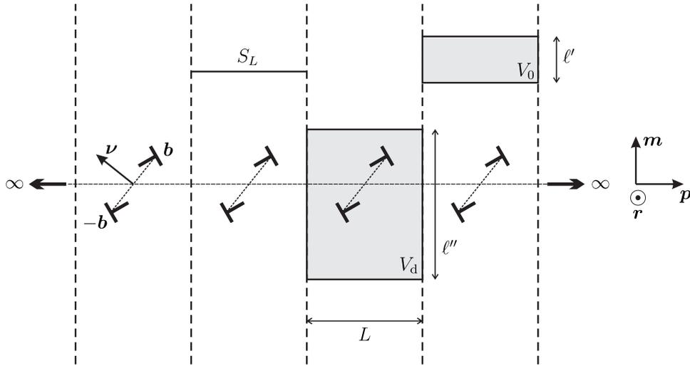
**Figure 3:** Periodic array (string) of dislocation dipoles. Two types of volumes are considered, both spanning exactly one period along the direction of periodicity: (i)  $V_0$  which is free of defects and (ii)  $V_d$  which contains the dislocation dipole.
