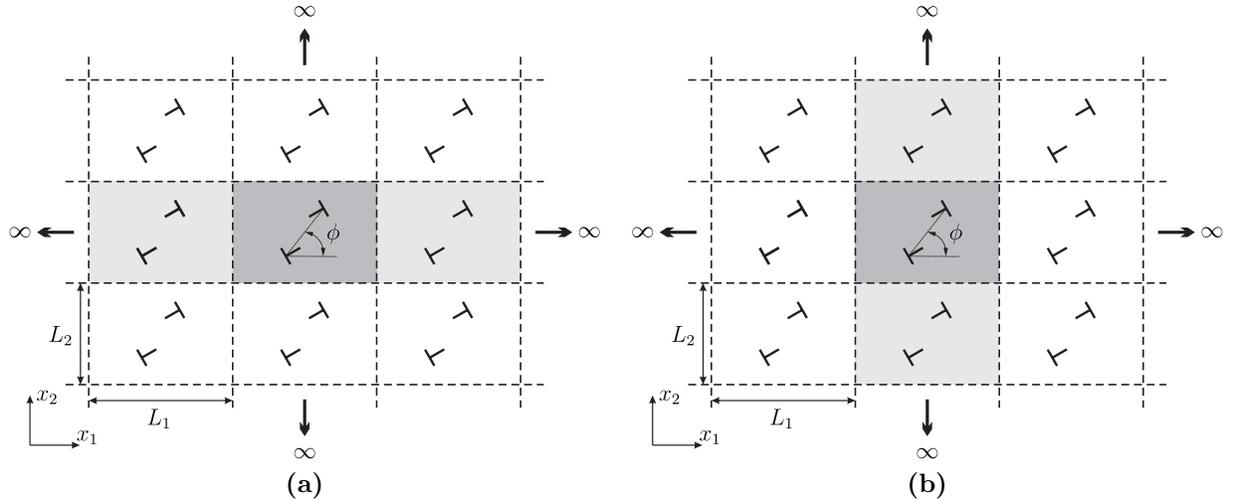
**Figure 4:** Doubly periodic array of dislocation dipoles: construction by superposition of (a) horizontal strings and (b) vertical strings. The primary strings employed in the superposition schemes are depicted in grey.
