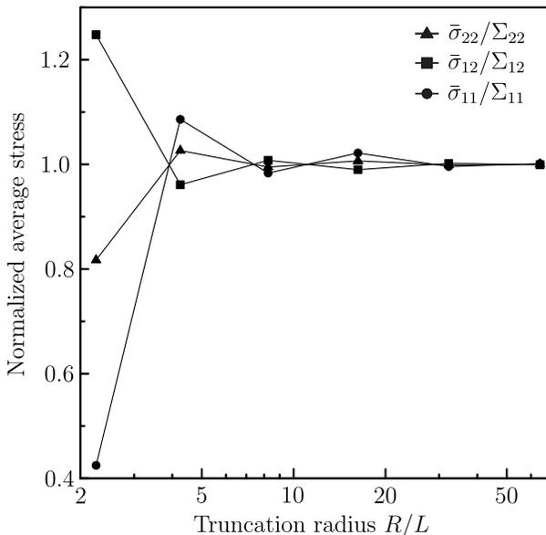
**Figure 6:** Convergence of the average stress  $\bar{\sigma}$  in the primary cell to the macroscopic stress  $\bar{\Sigma}$  determined from the Eshelby solution according to (62). The dipoles are characterized by the Burgers vector  $\mathbf{b} = (\sqrt{3}b/2, b/2, 0)$ , the slip-plane angle  $\phi = \pi/6$ , and distance  $d = L/6$ . The Poisson’s ratio of the material is  $\nu = 1/3$ .
