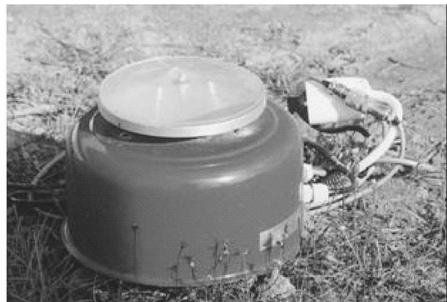
FIG. 2. Technical realization of the DBI impactometer. The quartz force sensor is used to measure the oscillations of the sensing plate originating from waterdrop impacts.
