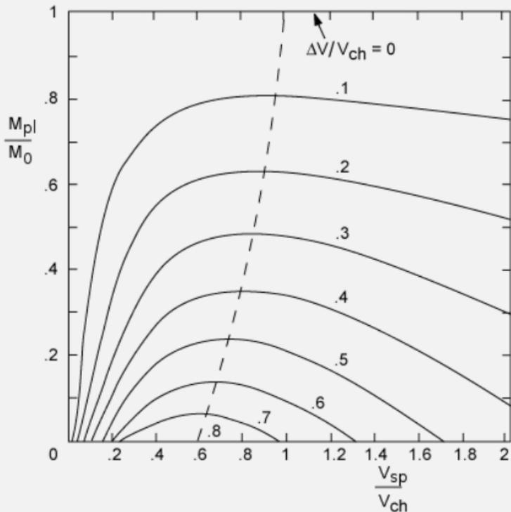
Payload fraction vs.  $V_{sp}$  for  $\Delta V \ll V_{ch}$
