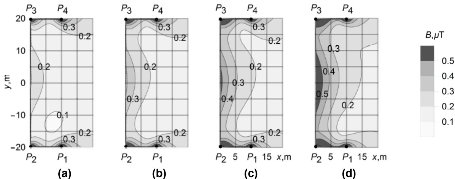
In Fig. (a)-(c) the grid shields reduce the magnetic field to 0.3–0.5  $\mu\text{T}$ .
