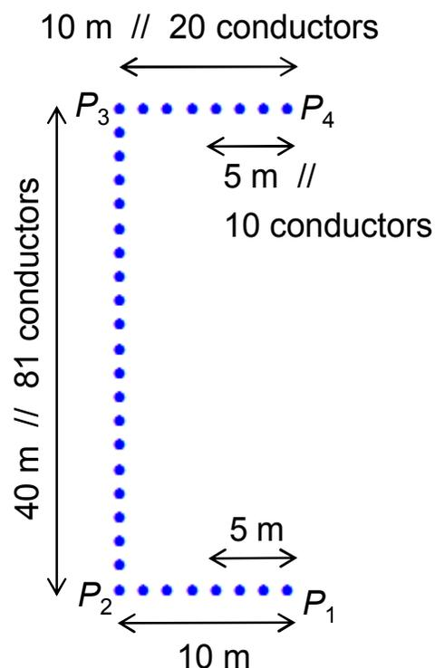
Cross-Section of Grid Shield
