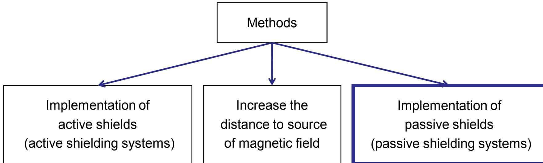
Active shield requires a source of electrical energy (to generate the current in its conductors), detectors and control system.
