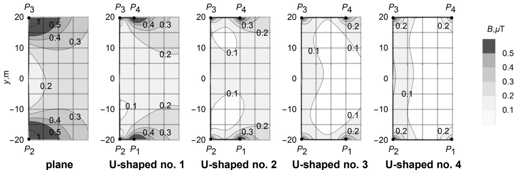
The shielded magnetic field  $B$  (in  $\mu\text{T}$ ) of the overhead line is shown with isolines. Each grey shaded region is limited by two isolines. The magnetic field varies from lower isoline value to higher one within corresponding region.
