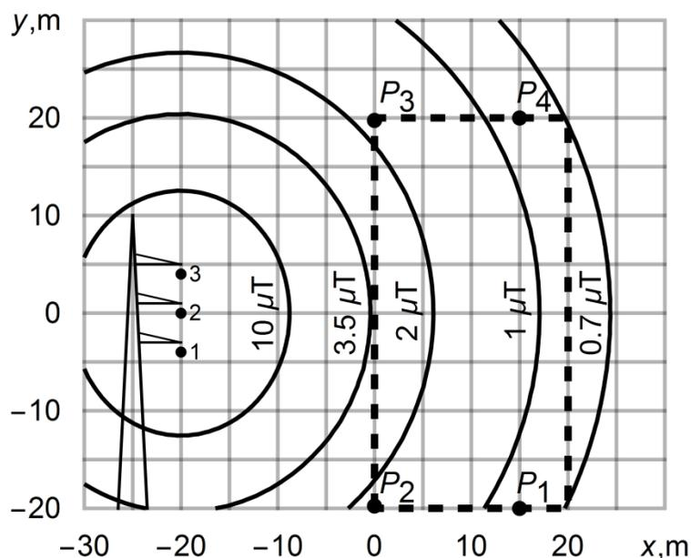
Points 1, 2, 3 indicate the conductors of OHL.
