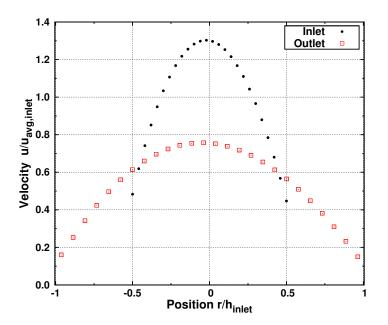
Fig. 4.6. Bended diverging channel flow; velocity profiles at inlet and outlet plane; both curves are normalised with inlet width h and average velocity; the *Knudsen* number is  $6.89 \cdot 10^{-2}$ .
