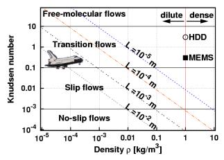
Fig. 6.1. Overview of flow regimes; the *Knudsen* number is shown in the function of density  $\rho$  and characteristic length scale *L*; flow situations for space shuttle on re-entry, flow between disk and head in a hard disk drive (HDD) and other micro-electro-mechanical systems (MEMS) are indicated.
