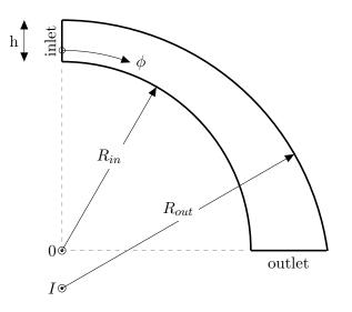
Fig. 4.3. Bended diverging channel setup; the radii are  $R_{in} = 5.5 \, 10^{-4} m$  and  $R_{out} = 7.5 \, 10^{-4} m$  with different midpoints; h is the inlet channel height defined as the characteristic length scale; the midpoint of angle  $\phi$  is point 0; the flow is from the inlet at position  $\phi = 0$  to the outlet.
