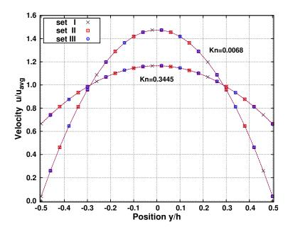
Fig. 3.5. Channel flow; normalised velocity at channel position x = 0.25 L, for two different *Knudsen* numbers Kn = 0.0068 (group 1) and Kn = 0.3445 (group 5) for nominally two-dimensional grid  $25 \times 125 \times 1.$
