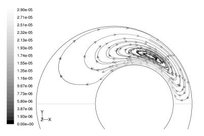
Fig. 4.8. Thermal stress slip flow stream lines; brightness corresponds to the velocity magnitude in [m/s];  $T_{in} = 300 \text{ K}$  and  $T_{out} = 320 \text{ K}$ ; axis of symmetry shown in lower part of the image; the *Knudsen* number is Kn = 0.0014.
