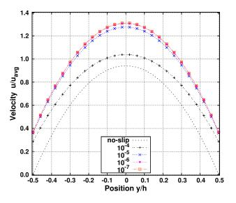
Fig. 5.5. Rectangular channel flow; velocity profiles at different convergence levels; all curves are normalised with the same average velocity from the  $\Delta_m = 10^{-7}$  level; the initial guess (no-slip) is plotted with a line only; the subsequent iteration levels are marked with point-lines; curves of convergence level  $\Delta_m = 10^{-6}$  and  $\Delta_m = 10^{-7}$  lie one over another.
