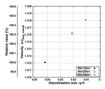
Fig. 5.1. Rectangular channel flow; normalised centreline velocities in the function of the discretisation size for three different grid levels at the stream-wise position x = 0.25 L; all values are normalised with the average velocity of the coarsest grid result  $u_{avg,coarse}$ ; the outer y axis shows the relative velocity difference referring to the coarsest grid result; the *Knudsen* number Kn=0.1 was chosen.
