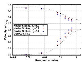
Fig. 3.7. Channel flow; normalised centreline (upper curve) and wall slip velocity (lower curve) in the function of *Knudsen* number for all groups in set I and nominally two-dimensional grid 25x125x1.
