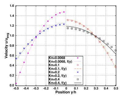
Fig. 3.6. Channel flow; normalised velocity profiles at channel position x = 0.25 L for four different *Knudsen* numbers (groups 1, 3, 4 and 6 of set I) for nominally two-dimensional grid 25x125x1. Only half of each profile is plotted to avoid overcrowding.
