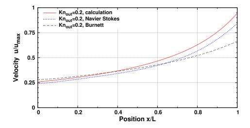
Fig. 3.4. Channel flow; wall velocity along the channel using the setup of set III; normalised with the maximum velocity at x = 0 position; curves are compared with results for *Navier Stokes* and *Burnett* equations [9].
