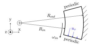
Fig. 3.9. Setup of Couette flow case; inner wall bounded by  $R_{in}$  is moving with rotational speed  $\omega_{in}$ ; the outer wall bounded by  $R_{out}$  is at rest.
