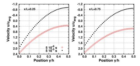
Fig. 3.13. Thermal creep setup; normalised x velocity distribution in the function of normalised channel height; left hand side labels indicate the streamwise x position (x/L = 0.25 and x/L = 0.75); curve symbols correspond to the simulation time for two different times  $t = 5 \, 10^{-6} s$  and  $t = 5 \, 10^{-5} s$ ; velocities are normalised with the average velocity of the x/L = 0.25 profile of the first time step; calculations were performed for average *Knudsen* number Kn=0.122
