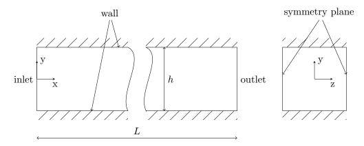
Fig. 3.1. Rectangular channel with length L and height h.
