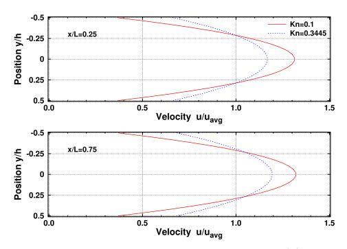
Fig. 3.2. Channel flow; velocity profiles at two positions along the channel (x/L = 0.25 and x/L = 0.75) for group 3 and 5 of set I; all velocities are normalised by the average velocity  $u_{avg}$  of the x/L = 0.25 profiles; the pressure ratio 1.05 was set.
