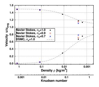
Fig. 3.8. Channel flow; normalised centreline (upper curve) and wall slip velocity (lower curve) in the function of density and *Knudsen* number (lower x-axis) for set II and nominally two-dimensional grid 25x125x1.
