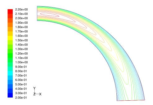
Fig. 4.4. Bended diverging channel flow; the colour scale indicates the normalised velocity magnitude; the *Knudsen* number is  $6.89 \cdot 10^{-2}$ .
