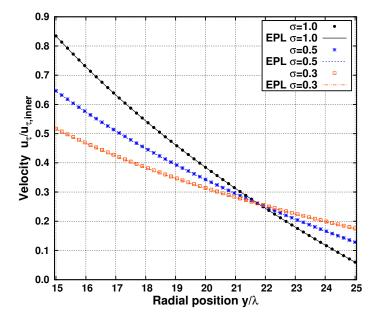
Fig. 3.10. Couette flow case; circumferential velocity  $u_{\tau}$  compared with the theoretical prediction from [7], labelled as EPL; the radial position is normalised by the mean free path  $\lambda$ ; result for nominally two-dimensional grid 60x52x1.
