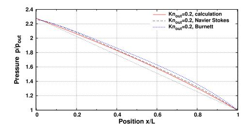
Fig. 3.3. Channel flow; pressure distribution along the channel using the setup of set III; values are normalised with the corresponding outlet pressure  $p_{out}$ ; curves are compared with results for *Navier Stokes* and *Burnett* equations [9]; additionally a straight line for  $p/p_{out}$  is plotted from inlet to outlet.
