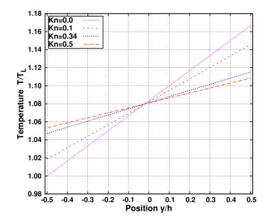
Fig. 4.2. Temperature jump boundary condition case; temperature profiles in the function of the normalised position for nominally two-dimensional grid  $25 \times 125 \times 1$  for four different *Knudsen* numbers.
