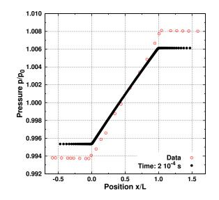
Fig. 3.15. Thermal creep setup; pressure distribution on horizontal plane located in the channel centre in the function of normalised x position; pressure is normalised with the ambient pressure  $p_0$ ; Kn=0.122; the comparison data are obtained from Direct Simulation Monte Carlo performed by [3].
