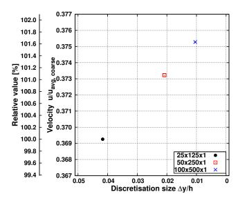
Fig. 5.2. Rectangular channel flow; normalised wall slip velocities in the function of the discretisation size for three different grid levels at the stream-wise position x = 0.25 L; all values are normalised with the average velocity of the coarsest grid result  $u_{avg,coarse}$ ; the outer y axis shows the relative velocity difference referring to the coarsest grid result; the *Knudsen* number Kn=0.1 was chosen.
