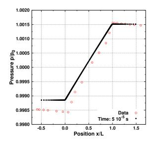
Fig. 3.14. Thermal creep setup; pressure distribution on horizontal plane located in the channel centre in the function of normalised x position; pressure is normalised with the ambient pressure  $p_0$ ; Kn=0.052; the comparison data are obtained from Direct Simulation Monte Carlo performed by [3].
