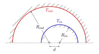
Fig. 4.7. Thermal stress slip flow setup; temperature at inner surface  $T_{in}$  is lower than outer surface temperature  $T_{out}$ ; d is the distance between the rotation axes; the dotted line indicates the symmetry plane.
