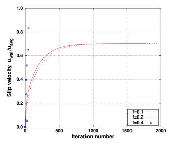
Fig. 5.7. Rectangular channel flow; normalised wall velocity in the function of iteration number for *Knudsen* number Kn = 0.4; all values are normalised with the average velocity  $u_{avg}$  of the f = 0.1 case result; the value of f represents different under-relaxation coefficients; for under-relaxation coefficient f = 0.4 or higher solutions do not converge.
