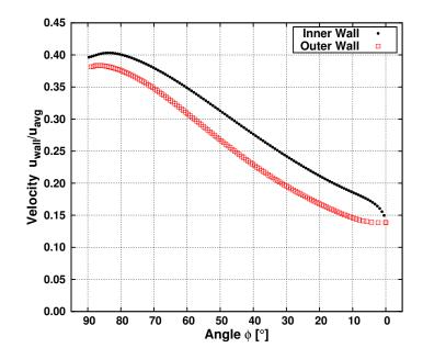
Fig. 4.5. Bended diverging channel flow; wall velocity normalised by the average velocity magnitude of the whole domain in the function of the arc angle  $\phi$ ; the *Knudsen* number is  $6.89 \cdot 10^{-2}$ .
