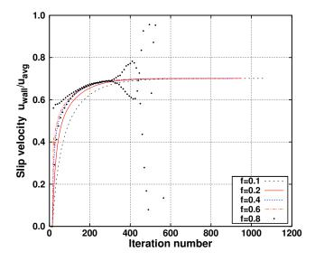
Fig. 5.6. Rectangular channel flow; normalised wall velocity in the function of iteration number for *Knudsen* number Kn = 0.1; all values are normalised with the average velocity  $u_{avg}$  of the f = 0.1 case result; the value of f represents different under-relaxation coefficients; it can be seen that all under-relaxation coefficients except f = 0.8 lead to convergent solutions.
