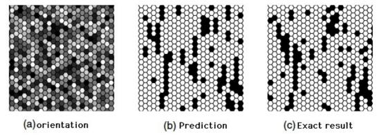
**Figure 1:** Example classification of polycrystalline microstructure. Orientation variation produces elastic property variation (a), classifier predicts location of stress concentration (b), finite element analysis provides validation result for classifier prediction (c).
