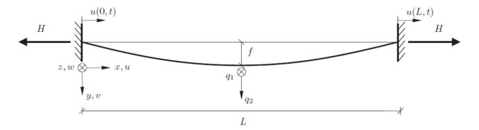
Figure 1. Cable in static equilibrium configuration.
