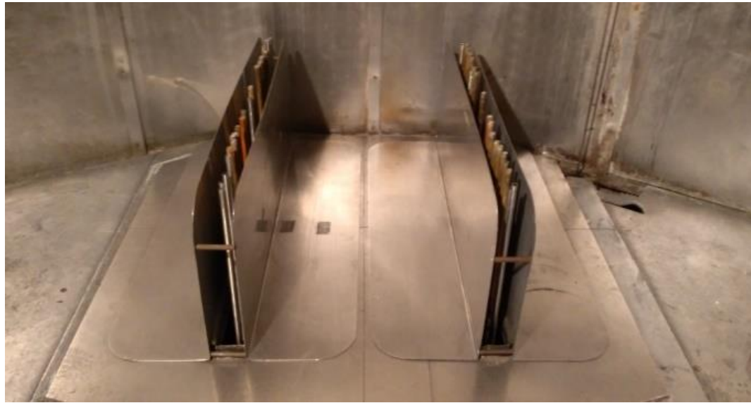
60 Co Irradiation chamber UGU-420 of the Joint Institute for Power and Nuclear Research – Sosny, Belarus
