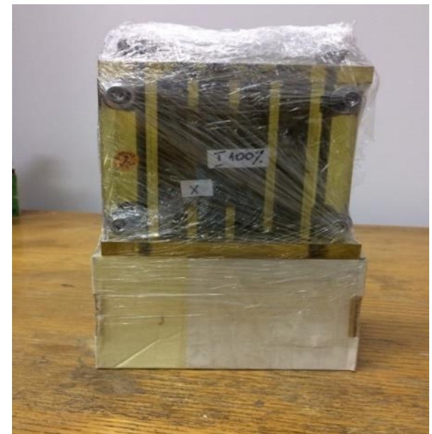
The mould with mortar wrapped against moisture lost
