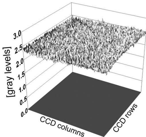
Fig. 1. Camera's  $3\sigma$  level at 200 ms exposure time.
