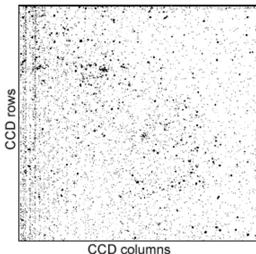
Fig. 4. Irregular cells. Due to representation limitations, the number of irregular cells seems to be higher than in reality (3 % of sensor area).
