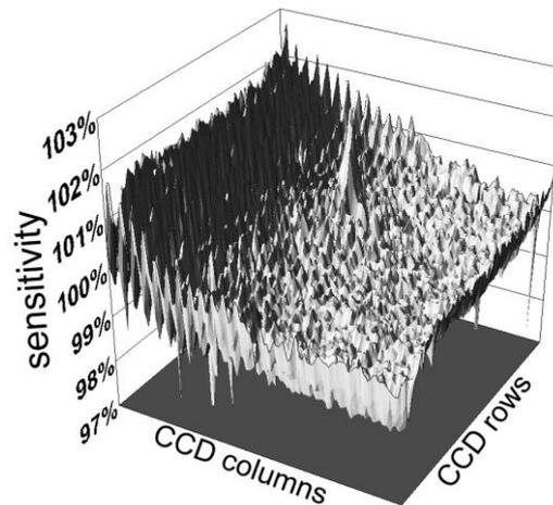
Fig. 3. Interpolated camera's sensitivity profile under dark conditions at 200 ms exposure time.
