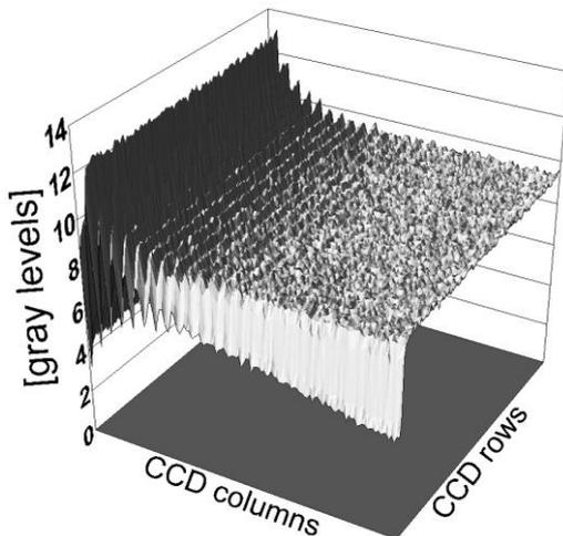
Fig. 2. Camera's dark profile at 200 ms exposure time.
