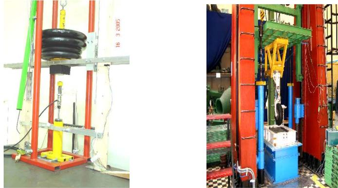
**Fig. 14** Developed lab scale drop test stand (left) and full scale drop test stand (right)
