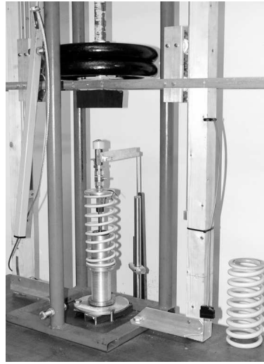
Figure 17: (left) Laboratory model of Adaptive Impact Absorber (AIA); (right) AIA mounted on the laboratory drop test rig
