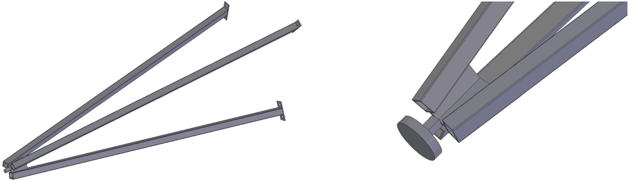
Figure 2. Truss construction without and with the additional mass
