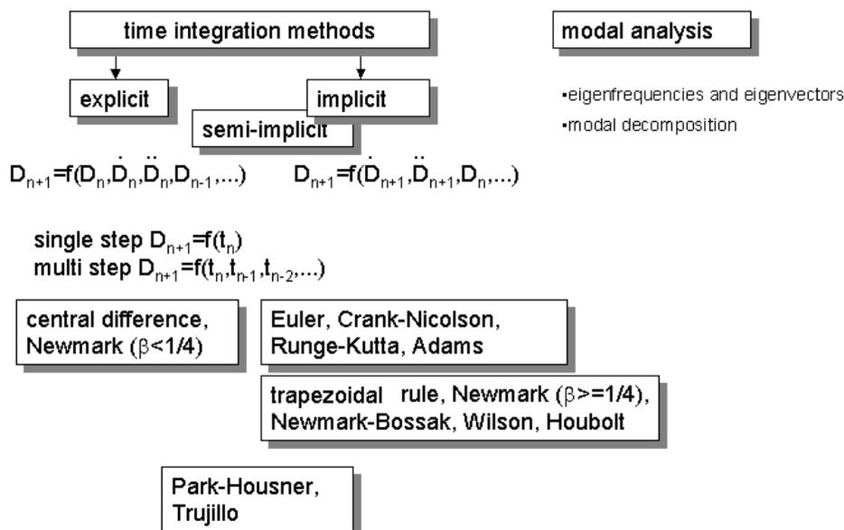
Fig. 1. Numerical methods employed in structural dynamics.
