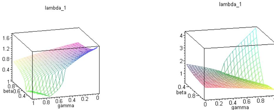
Fig. 2. Spectral radius of the transfer matrix for Newmark method.
