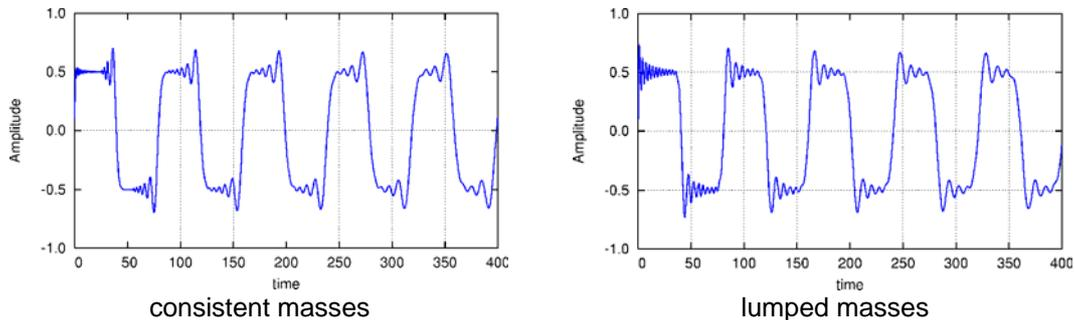
Fig. 8. Artificial damping effect with constitutive and lumped mass matrices.
