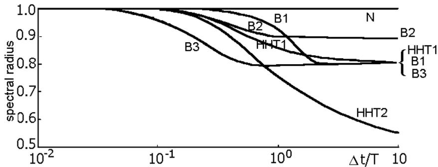
Fig. 3. Spectral radius for selected time integration methods [2].
