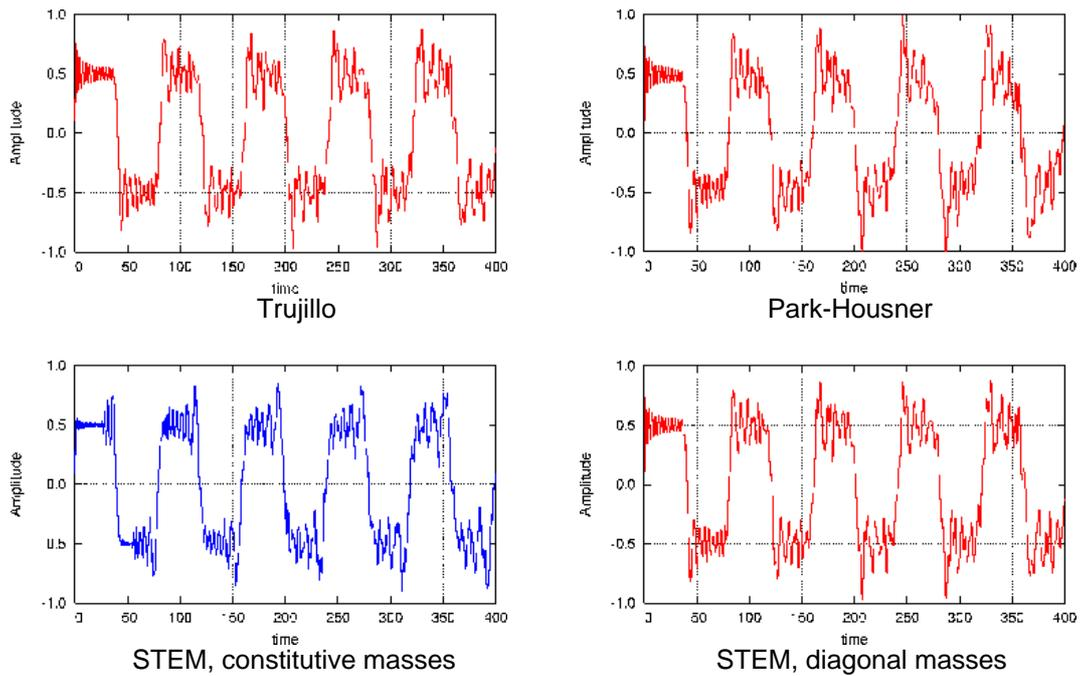
Fig. 7. Vibrating bar solved by different methods (no damping).
