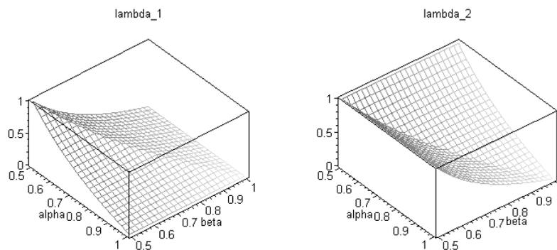
Fig. 4. Spectral radius of the transfer matrix for Park-Housner method.
