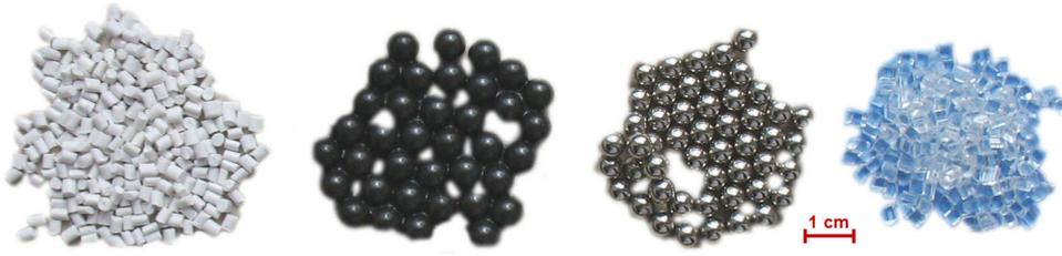
**Figure 2.45.** Types of the tested granular materials, from the left: plastic rollers, plastic spheres, steel spheres and plastic cubes.
