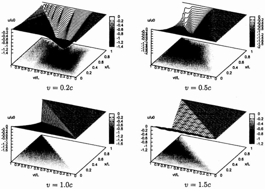
Figure 4: Simulation of the string motion under the mass moving at  $v=0.2c$ ,  $0.5c$ ,  $1.0c$  and  $1.5c$ .
