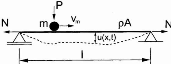
Figure 1: A string under the moving mass.
