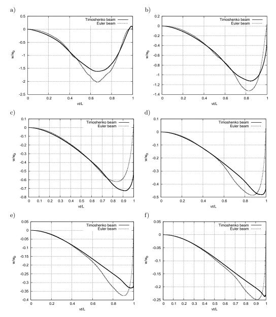
Fig. 6. Trajectory of a mass travelling at the speed: a) v=0.1, b) v=0.2, c) v=0.3, d) v=0.4, e) v=0.5 and f) v=0.6 ( $c_1=0.63$ ,  $c_2=1.00$ ).
