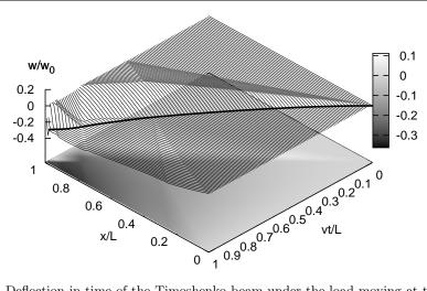
Fig. 4. Deflection in time of the Timoshenko beam under the load moving at the speed  $v=0.5c_2$ .
