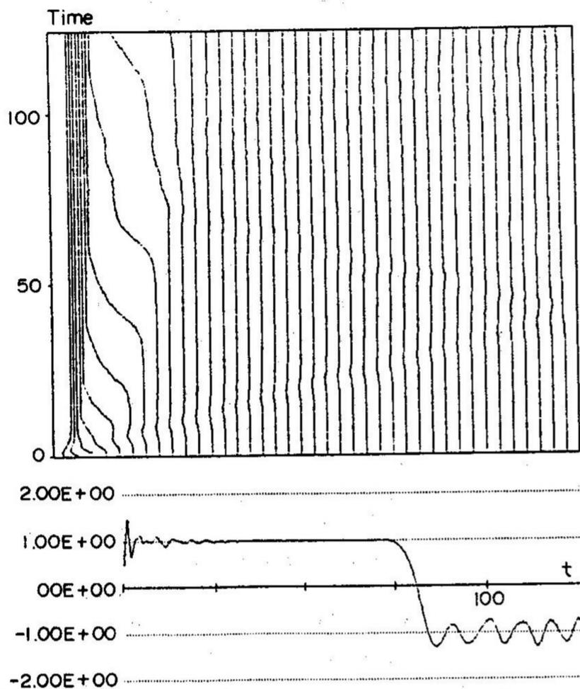
Fig. 6. Mesh evolution in the bar subjected to an impulse placed at the end.
