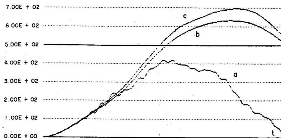
Fig. 9. Displacements in time assuming (a) deflectional error estimator, (b) rotational error estimator, (c) constant spatial partition.
