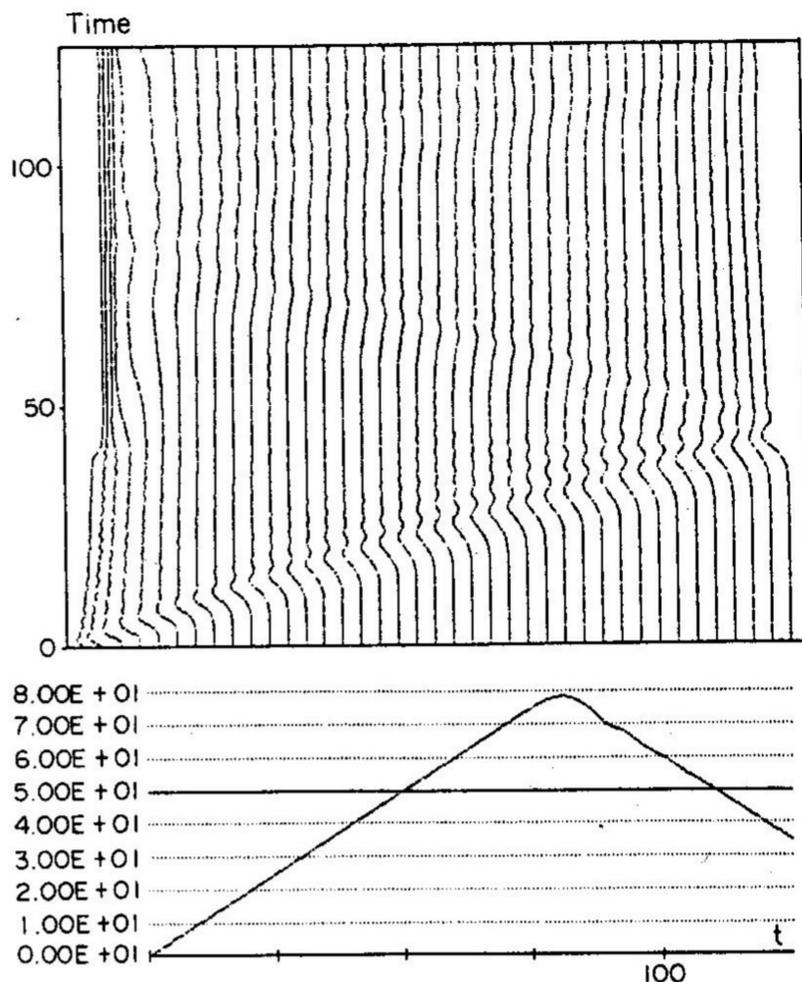
Fig. 7. Mesh evolution in the bar subjected to a Heaviside load placed at the end.
