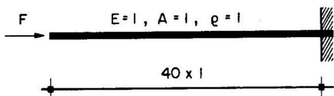
Fig. 5. Axial vibration of a bar—sample problem.
