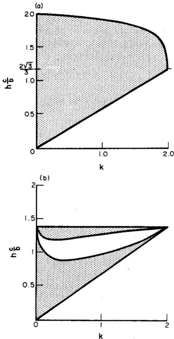
Fig. 3. Stability domain for quadrangular and triangular bar elements.
