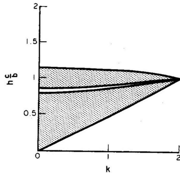
Fig. 4. Stability domain for tetrahedral plane strain elements.
