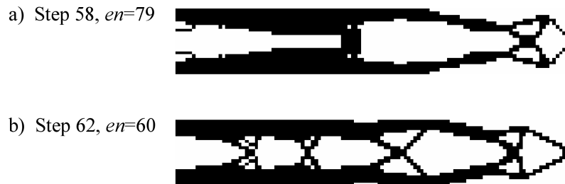
Fig. 13. Topologies for p = 1 , a = 1000 and \alpha = 0.5 , obtained using Alg-1 a) and Alg- b)
