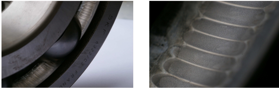
Fig. 3. Bearing race damages caused by EDM currents
