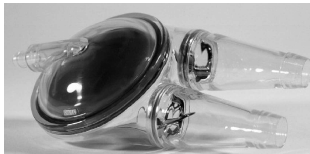
Fig. 2. Polish heart-supporting device – POLVAD after Ref. [11]
