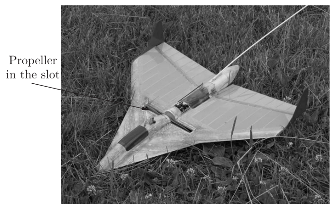
Fig. 2. Possible design of gust resistant fixed wing MAV
