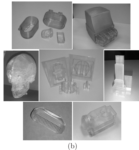
Fig. 5. Diagram of model creation by (a) stereolithography and (b) a manufactured products
