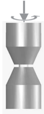
Fig. 3. Scheme of the HPT process
