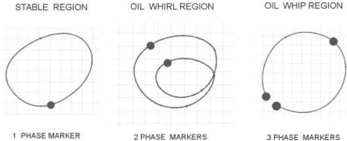
Fig. 12. Proposed classification of hydrodynamic instabilities in the system and introduction of diagnostic determinants
