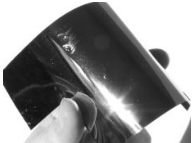
Fig. 8. Test structure of elastic CdTe layer based on UPILEX® foil and contacted by 2µm Cu layer
